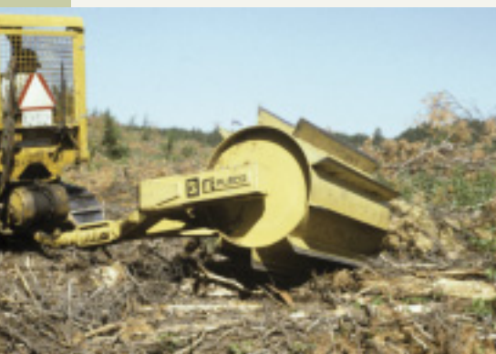
A drum chopper can be used to help breakdown logging slash and debris.
