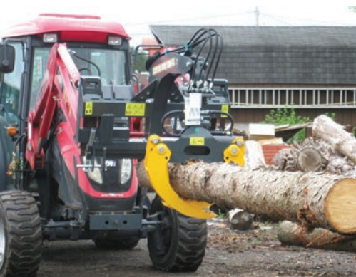
Figure 12. Grapples are also made for tractors but require the tractor to backup to each log.
