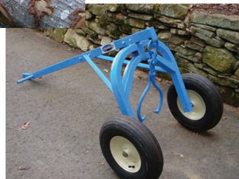
Figure 5. Some arches use tongs to grab logs while others use cables and chains.
