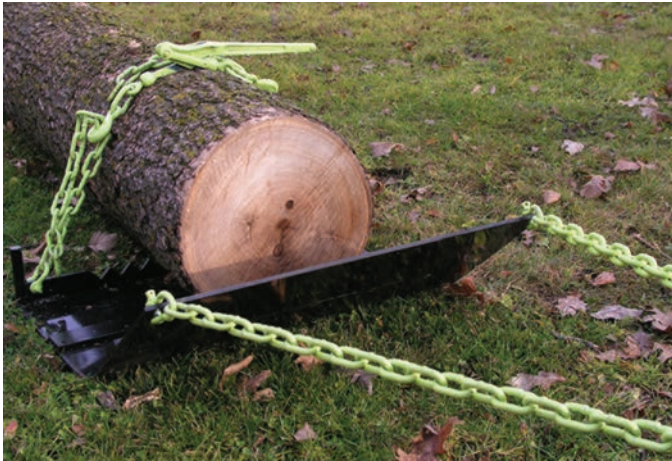
Figure 1. A skidding plate is the least expensive attachment for safely skidding with a four wheeler.
