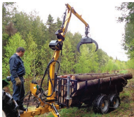
Figure 8. Trailers are an efficient means of moving smaller logs, poles and firewood.
