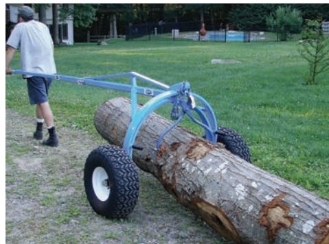
Figure 4. Some arches can be pulled by hand and by four wheelers.
